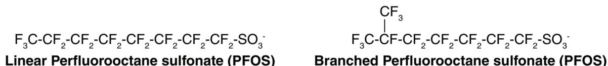
**Figure 4-1. Linear and one branched isomer of PFOS**
